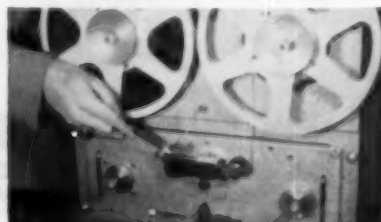
Fig. 2. Pencil points to the spot on the back of the tape which has been moved back directly over the erase head prior to putting the machine in the record mode. Again white leader tape is used so that it will show up against black head assembly.
