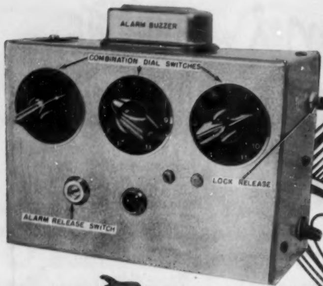
Fig. 1. Although the author's unit, as shown above, employs only three dials any number can be added for greater safety.
