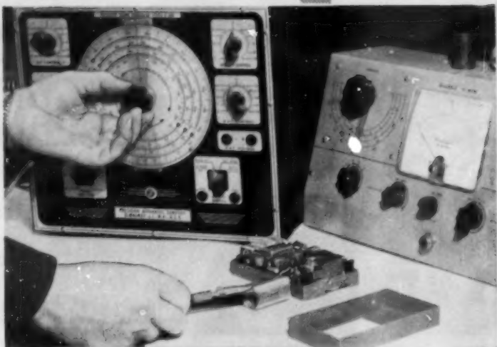
Fig. 1. To inject signal and i.f. frequencies into transistor amplifier stages, use an inductor as shown with a.c. operated generators. Battery-operated signal generators will be found useful for transistor testing in audio and signal stages.
