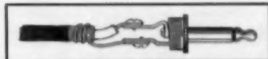
Fig. 2. Shown here is the correct way to connect single conductor, shielded cable to a microphone plug. Note that the shield is not brought to the screw.
