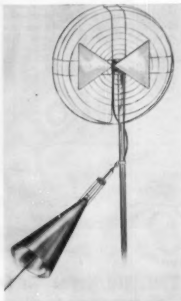
Fig. 1. View of the launchers used at the antenna and house end of the "G-Line." The wire itself is strung directly from the antenna to the house entrance of the lead-in wire; the launcher sends the received signal down the wire in the method peculiar to this type transmission line.
