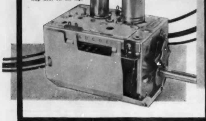
Fig. 1. Exterior of the new turret tuner. Note the solder terminals on the side and top and the covered trap door on the top.
